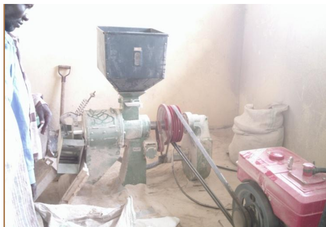
The rice huller machine in operation at social welfare project at Namehere village in Butaleja.
